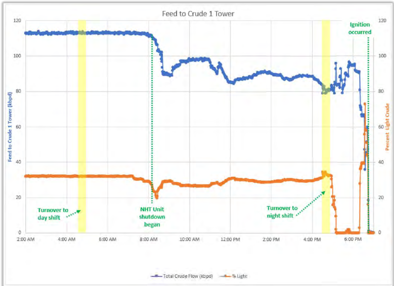
Figure 22: Crude 1 Tower Feed rate (blue) and percent light feed composition (orange) day of incident. The yellow bars indicate shift change turnover. (Credit: CSB)
